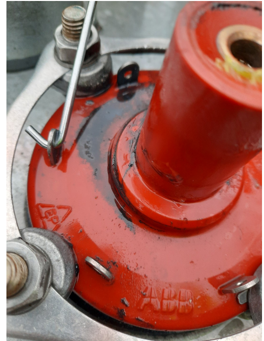
Image 2. The broken transformer bushing at the facilities of E.ON Sweden.
